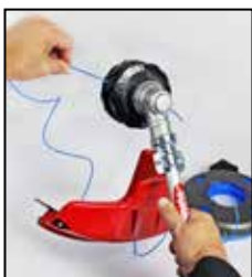
2. Feed the trimmer line through the head
