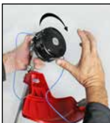
4. Twist head "clockwise" until ~8" trimmer line shows
