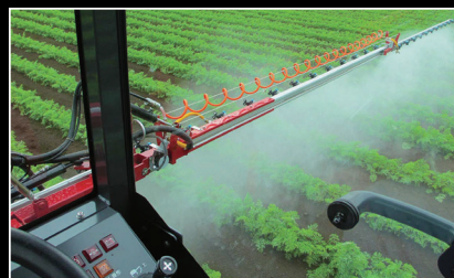
FORWARD COCKPIT Full 180° view with forward visibility to adjust speed and to verify nozzle performance
