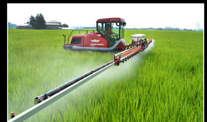
MID-TANK LAYOUT Located in the center of the spray tractor. The weight balance between the front and the back is constant allowing for driving stability even in wet fields
