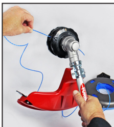
2. Feed the trimmer line through the head
