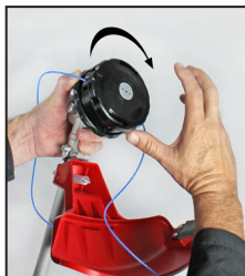
4. Twist head "clockwise" until ~8" trimmer line shows
