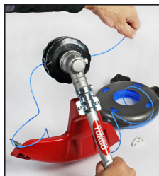
3. Pull line through* - make both sides equal lengths
