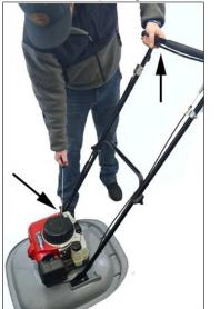
e. Pull the starter rope out slowly about 6-8" before beginning the full pulling motion and do not pull it all the way out. After the engine has started, move the choke lever to the OPEN position, then carefully move behind the unit while continuing to hold the stop lever against the handle and adjusting your grip position using **both hands**.
