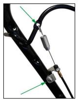
7. The throttle cable MUST be adjusted after installation.
