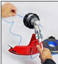
2. Feed the trimmer line through the head
