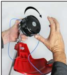
4. Twist head "clockwise" until ~8" trimmer line shows
