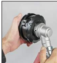
1. Line up the arrow on the head with the eyelet
