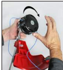
4. Twist head "clockwise" until ~8" trimmer line shows
