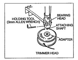
Note: Use 3mm allen wrench (from tool kit) as a holding tool to lock the attaching shaft while installing cutting devices (see sketches).
