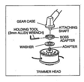
Install the trimmer head, as shown. Be sure the trimmer head is for LEFT-HAND rotation (as viewed from the operator's position) and the trimmer head adapter matches the internally-threaded splined attaching shaft of the tool (M8 x 1.25 LEFT-HAND).
