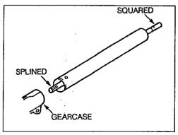
Insert the driveshaft tube assembly into the cultivator gearcase assembly while rotating the driveshaft to engage the splines.
