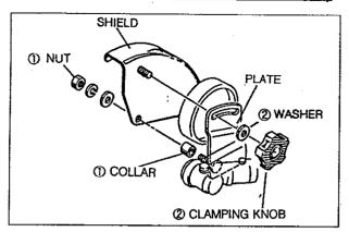
Nip the collar as sketched and fix the shield and the plate with nut and washers (1), and then with clamping knob and washer (2).
