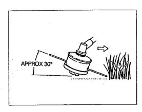
that exceeds the capability of the machine (Continuous overload may cause damage to the machine). Whenever grass or debris winds onto the shaft or trimmer head, immediately stop the machine and remove the interfering material.
