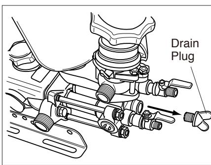
Water should be completely drained during winter storage to prevent freezing. The operation is performed according to items from 11 to 18 in the operation procedure.
