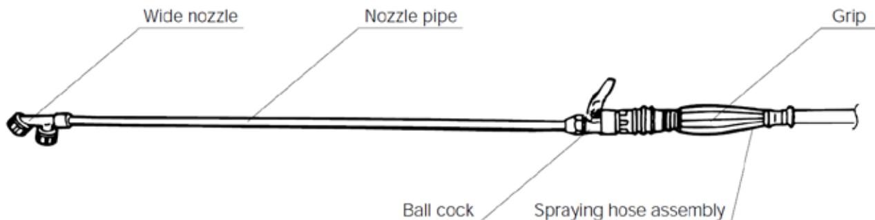
After confirming the existence of packing, securely tighten nozzle pipe to grip, and wide nozzle to nozzle pipe. Tighten the screw securely after confirming the packing to make ensure there is no water leakage. Over-tightening will cause extrusion or break the packing. Correct tightening pressure is important.
