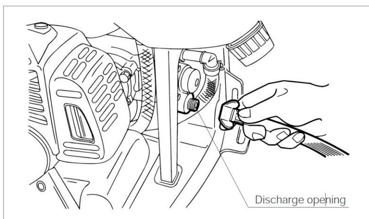
Connect opposite side of hose to discharge opening of the spraying machine.
