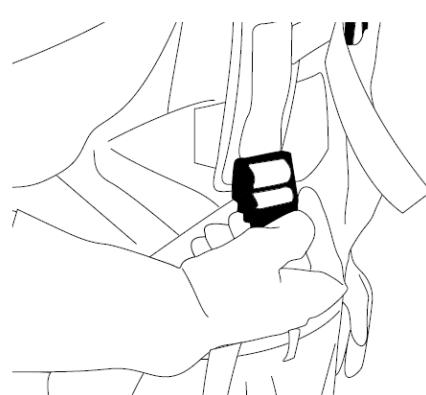
Lift strap buckle upward to loosen.
