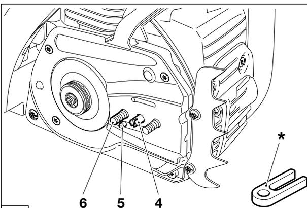
Remove the plastic transport cover (\*) and dispose of properly.
