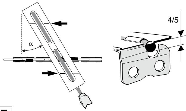
A file holder makes file guidance easier. It is marked for the correct sharpening angle of:
