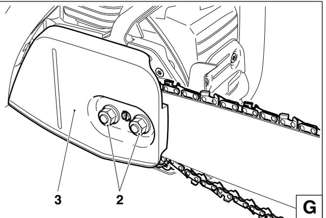
**Tightening the saw chain**
