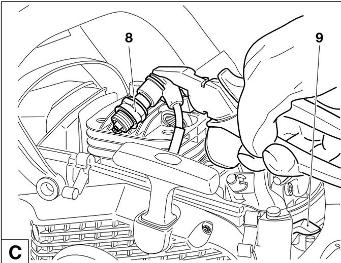
With the spark plug removed and the spark plug cap firmly seated, use insulated pliers to hold the spark plug (8) against the cylinder (not the spark plug hole).
