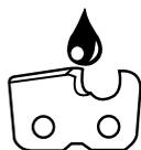
Use an oil with adhesive additive for lubricating the chain and guide bar. The adhesive additive prevents the oil from being flung off the chain too quickly.
