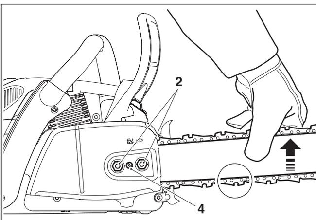
**Tightening the saw chain**
