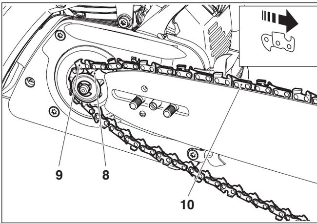
Lift the chain (9) over the sprocket (8).
