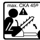
Maximum Computed Kickback Angle (CKA)\* without using the chain brake when using the recommended bar and chain combinations (In this example the CKA is 45°).
