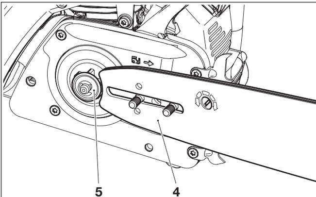
Put the guide bar (4) on and push it against the sprocket (5).
