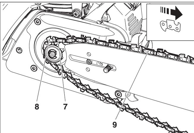
Lift the chain (8) over the sprocket (7).
