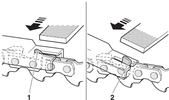
After having sharpened the chain, the height of the depth limiter must be checked by means of a chain gauge. See „Accessories“ for the order number.
