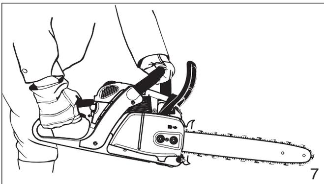
Wrap your fingers tightly around the handles, keeping the handles cradled between your thumb and forefinger (fig. 7). With your hands in this position, you can best oppose and absorb the push, pull and kickback forces of your saw without having it slip out of your grip (see section of reactive forces). Make sure your chain saw handle and grip are in good condition and free of moisture, pitch, oil or grease.
