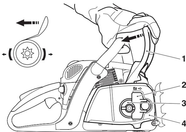
**Mounting the guide bar and saw chain**
