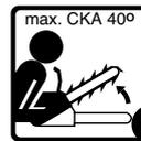
Maximum Computed Kickback Angle (CKA)\* with using the chain brake when using the recommended bar and chain combinations (In this example the CKA is 40°).
