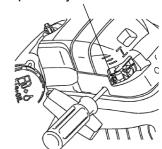
To adjust the engine idle speed, rotate the idle speed adjustment screw on the carburetor.
