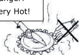
**If a foreign object, such as a piece of wire becomes tangled in the Landscape Blade stopping blade rotation, stop the engine first before removing the object. If blade rotation is still not smooth after removing the object, see the "Maintenance" section of this manual (Page 8) for further troubleshooting information.**
