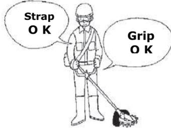
Adjust the shoulder strap and grip position, so that the blade face is parallel to the ground.
