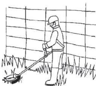
Grass close to a wall, solid fence or tree can be easily trimmed with minimal damage because of blunt edged blades and minimal back because the blades counter rotate.
