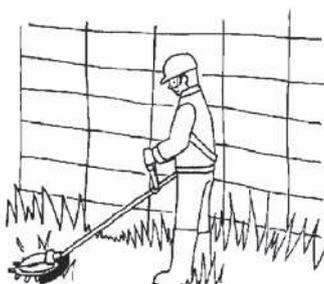
Grass close to a wall, solid fence or tree can be easily trimmed with minimal damage because of blunt edged blades and minimal back because the blades counter rotate.
