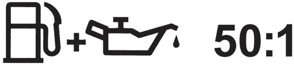
**Note:** Never use a mixing ratio less than 50:1 regardless of the oil package mixing instructions. Ratios less than 50:1, (for example, 60:1, 80:1, 100:1), reduce the amount of lubrication to the internal moving parts of the engine and can cause damage.
