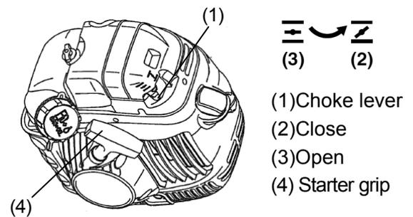
4. While holding the unit firmly, pull out the starter grip quickly until engine started.
